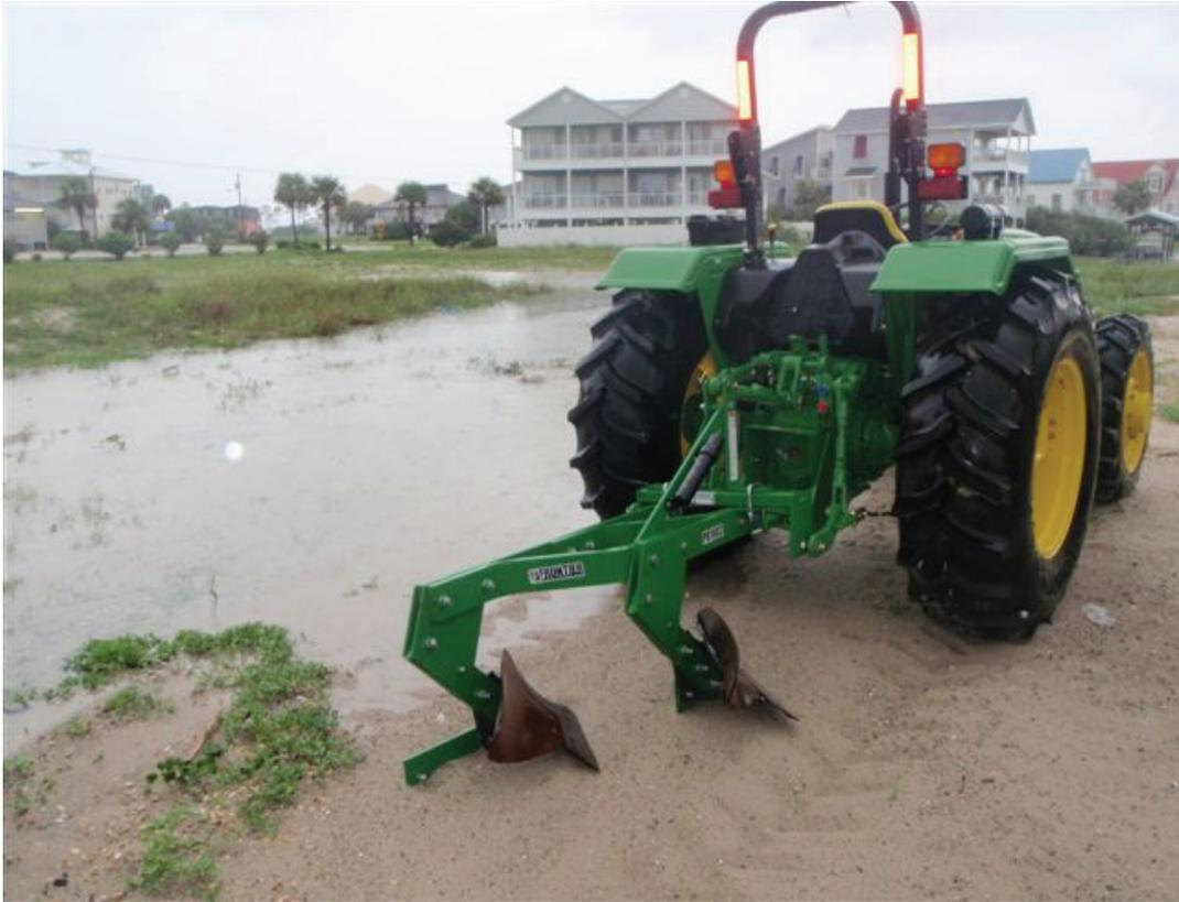
**Figure 5.28** Shallow to Moderate Depth Mixing by Agricultural Plowing
